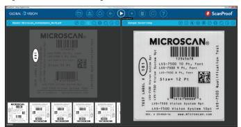
The PDF Comparator is an optional advanced error detection program for the LVS-7510 which compares one reference "golden image" to a PDF master artwork file selected by the user. The PDF Comparator compares the approved master artwork file to the golden image, and the Blemish Detection Tool compares the golden image to the rest of the labels.
